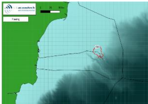
Figure 6.89 Cumulative impulse noise exposure level for fish (Popper et al., 2014) with the hammer in the best scenario for the installation of four successive piers, the outer isoline is the TTS limit and the inner one \geq 203 dB
