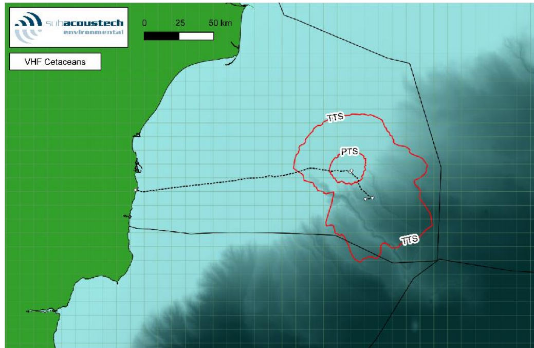
Figure 6.108 SEL cumulative pulse noise exposure level (Southall et al., 2019) species Phocena phocena with the hammer used at optimal energy for the installation of 4 piles, the inner isoline is the PTS limit and the outer isoline is the TTS limit
